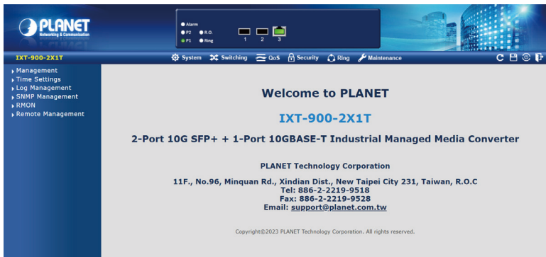
Figure 2. Web Main Screen of Industrial Managed Media Converter (Use IXT-900-2X1T as a representative)
